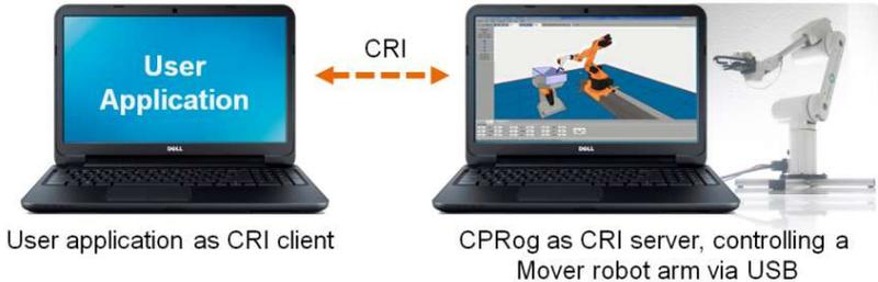
This interface makes it possible to combine the CPRog functions with application-specific algorithms, such as a teleoperation system or a database.
