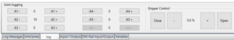
Figure 5: The buttons for joint movements. In the card safe mode, the keys change to X, Y, Z, A, B, C.
